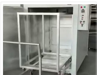
Trolley positioned at the oven
