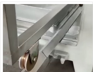
Rack engaged with the oven system
